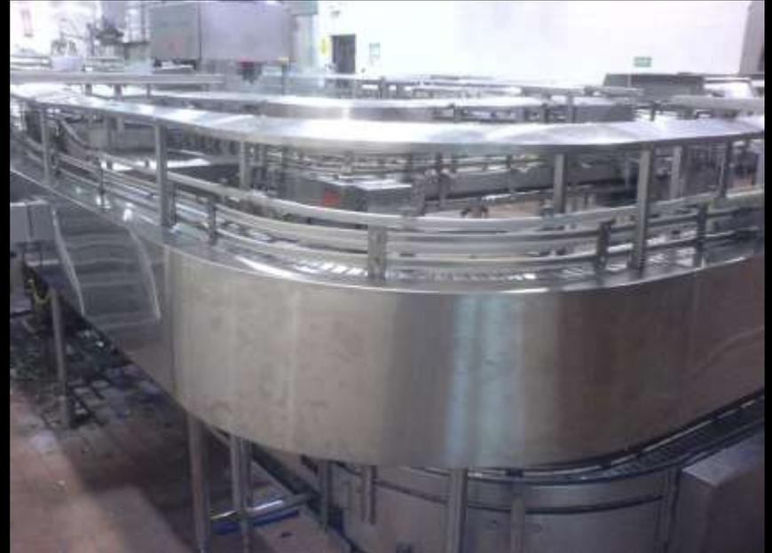
ELIMINAR TRASLAPE Y FABRICAR E INSTALAR CURVA, CON FALDÓN Y CUBRE POLVO.
